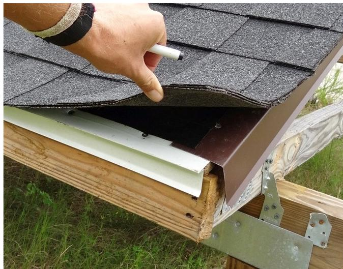
**Fig. 114. Pull-through of the starter strip around fasteners on LAM-201 – Roof 2. The fasteners were placed approximately 127 mm (5 in) from the butt edge of the starter strip.**
