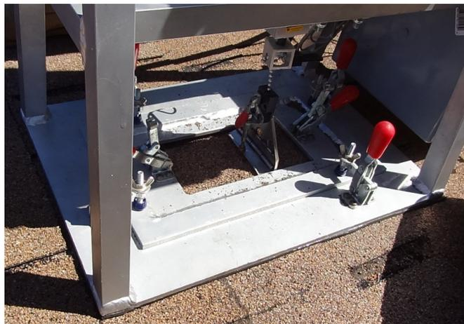
Fig. 31. The Portable Test Apparatus performing in-situ ASTM D6381 Procedure A mechanical uplift tests.
