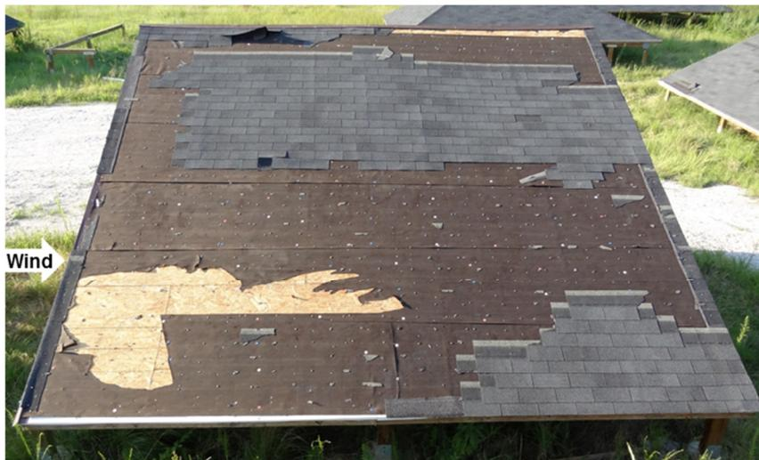
**Fig. 129. TT-201 - Roof 3 with blown off shingles caused by eave and rake shingles that pulled-through their edge fasteners. Note: The location of fasteners was not within ARMA (2006) specification.**
