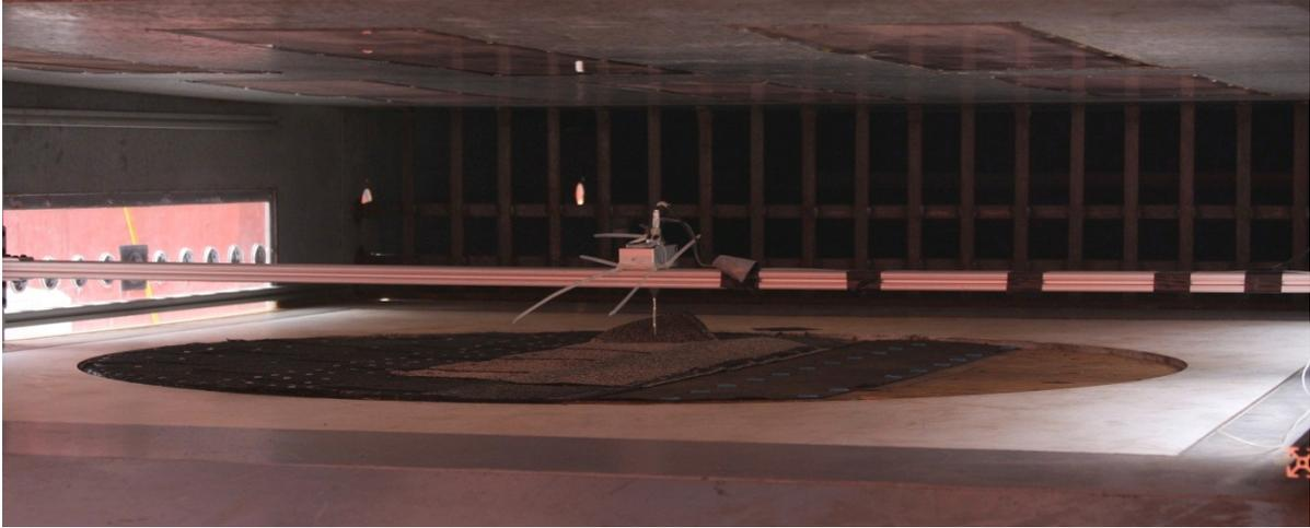
**Fig. 57. Test specimen in the Dynamic Flow Simulator test section with upstream turbulence grid shown.**
