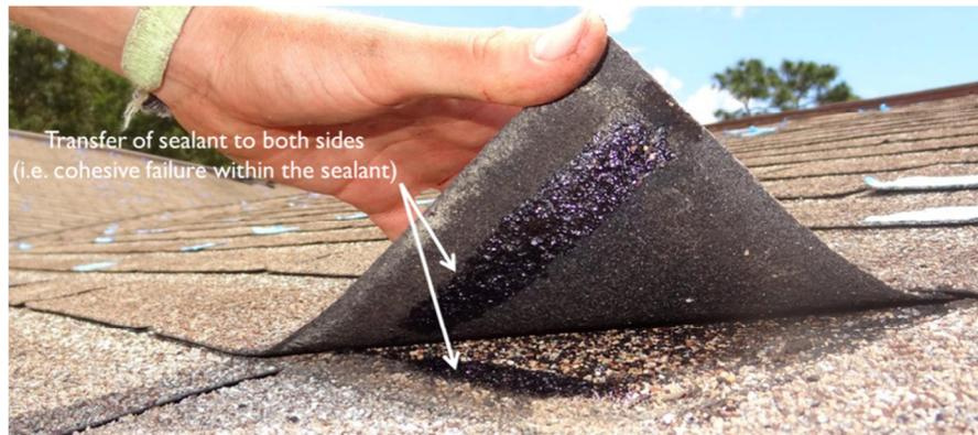
**Fig. 41. All unsealed shingles near the end joint failed cohesively within the sealant strip, suggesting that shingles were previously adhered.**
