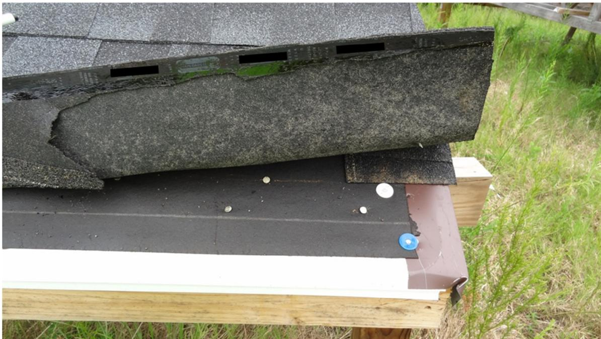
**Fig. 122.** Pull-through of the shingle system’s eave starter strips around the fasteners on LAM-202 – Roof 2. The fasteners were placed approximately 127 mm (5 in) from the butt edge of the starter strip.
