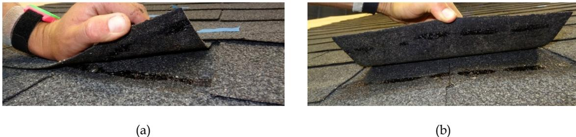
**Fig. 123. TT-201 – Roof 5 pre-test unsealing was caused by a cohesive failure in the tab sealant for both (a) partially and (b) fully unsealed shingles.**
