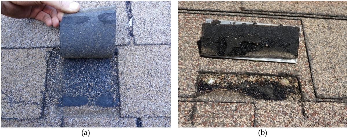
**Fig. 32. Example of failure modes for mechanically uplifted shingles: (a) cohesive failure in the adherend (ORM-01) and (b) combined cohesive failures in the sealant and adherend (ORG-01).**
