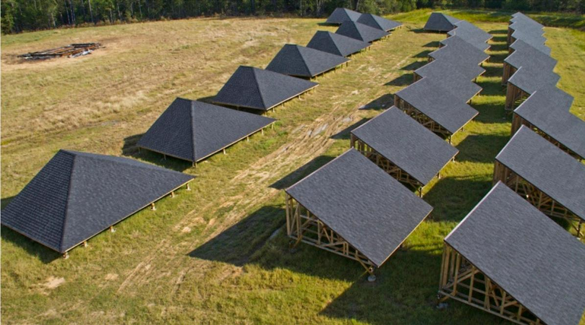
**Fig. 98. Aerial view of the completed asphalt shingle roof sections at the IBHS Research Center. The roofs were located at this field site throughout their 11 month conditioning phase.**
