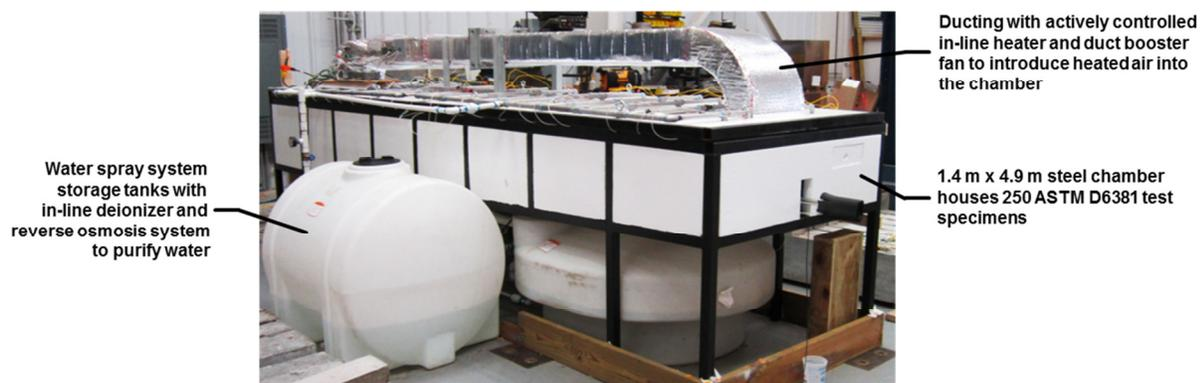
Fig. 21. Exterior view of the accelerated aging chamber.
