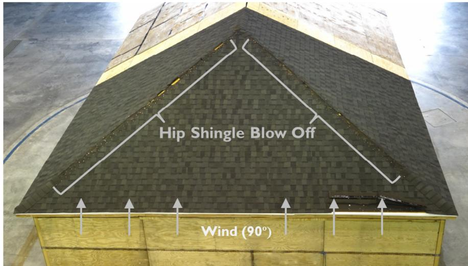
**Fig. 135. Typical hip shingle blow off for 90° wind azimuth (photo of LAM-201 – Roof 6 specimen).**
