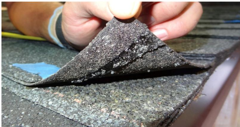
**Fig. 119. Pre-wind test unsealed rake shingle with an adhesive failure mode – LAM-202 – Roof 3.**
