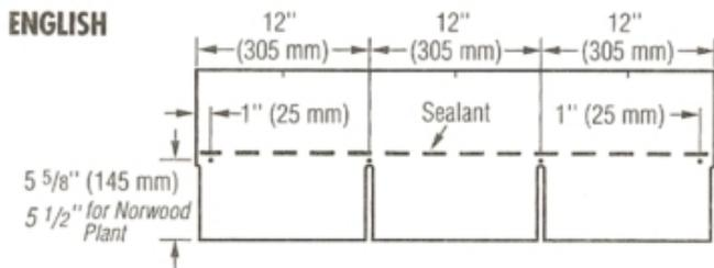
The dark dashed line in this drawing of a conventional three-tab shingle is the asphalt sealant strip.
